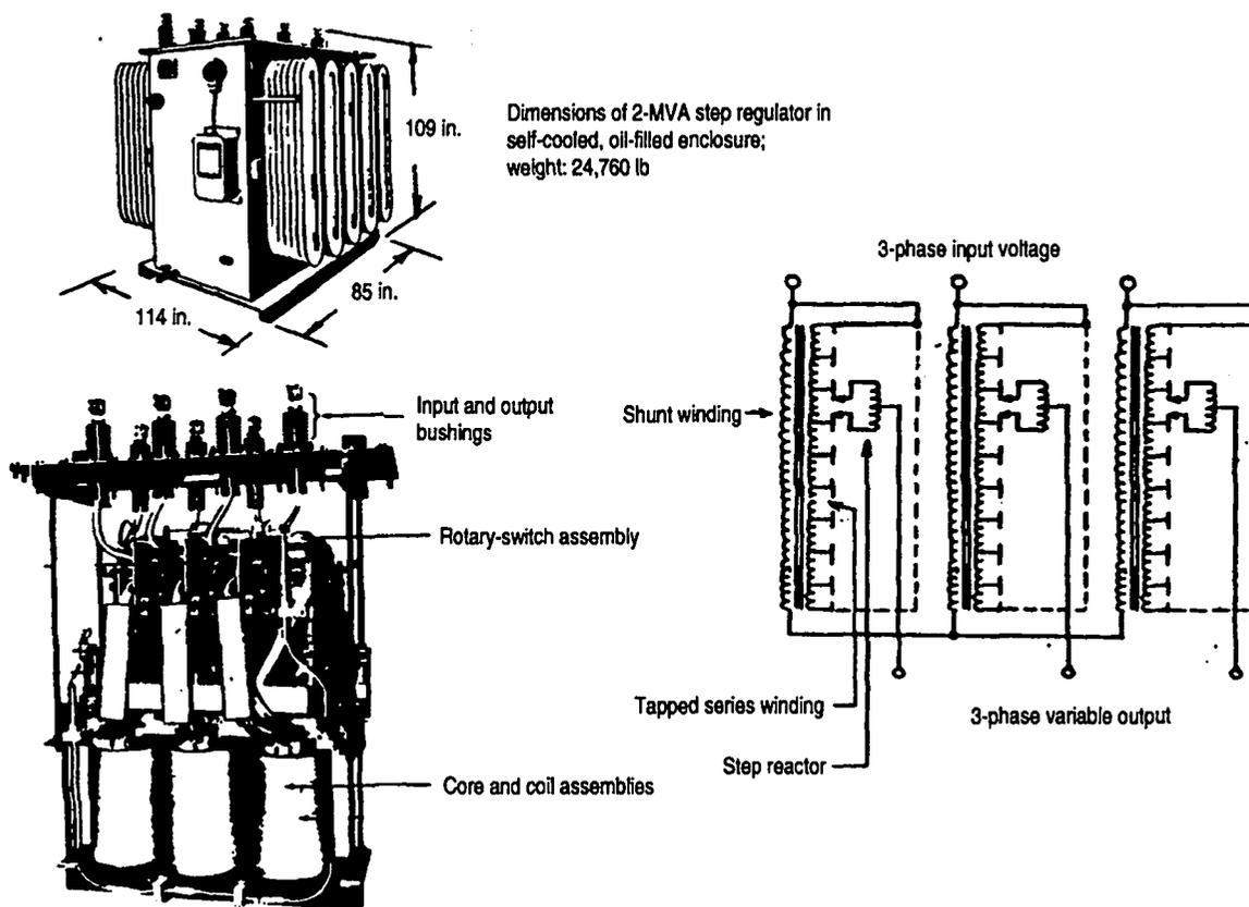
Figure 15-10. The 32-step (16 buck and 16 boost) voltage regulator.
