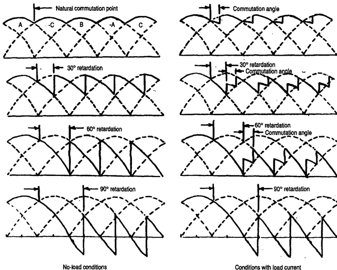
Figure 15-2. Phase-controlled rectifier waveforms for different output voltages.
