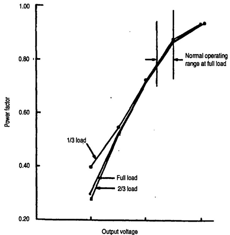
Figure 15-6. Effect on input-power factor as output voltage is varied.
