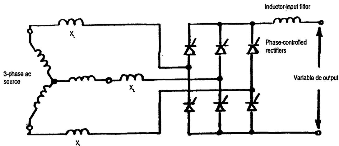
Figure 15-1. The phase-controlled rectifier variable-output dc power supply.
