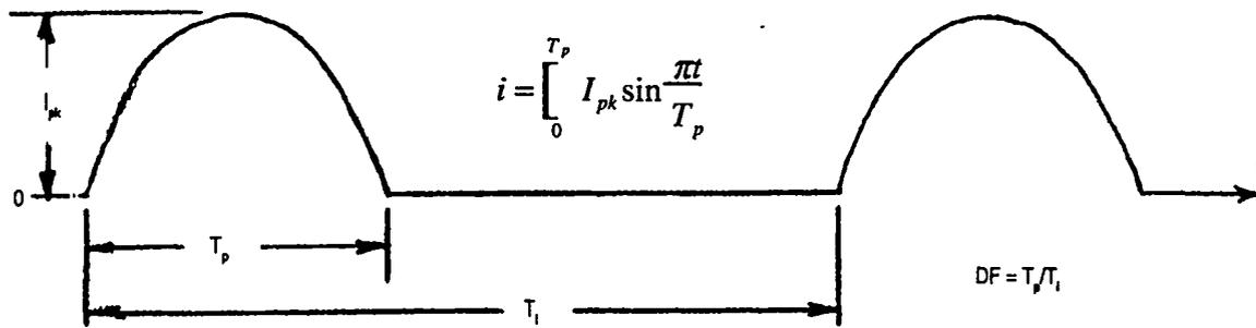
Figure 6-3. Recurrent rectified sine wave.
