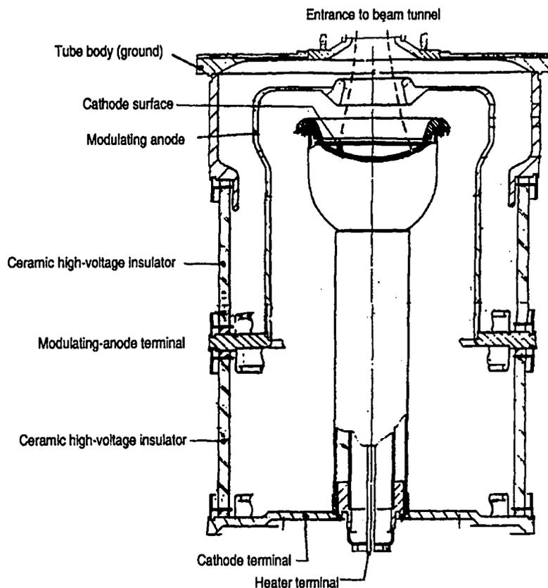
Figure 8-2. High-power microwave-tube electron gun with modulating anode.
