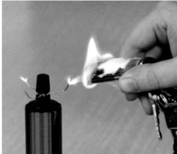
**Figure 11.** The heat contained in an rf discharge can be quite intense, although the skin effect defends against risk of electric shock.
