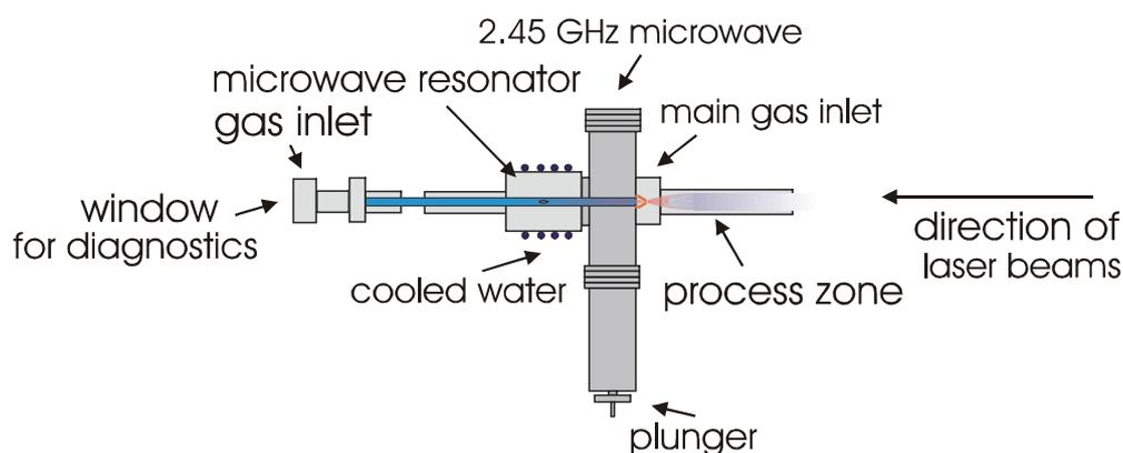
Figure 1: Experimental arrangement.
