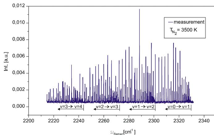
Figure 4: Measured CARS spectrum at the center of the microwave discharge. Experimental data of several hot bands together with their rotational lines are shown. The spectra delivers a gas temperature of 3500 K at 800 W microwave power.
