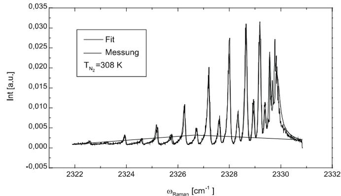
Figure 3: CARS spectrum (Q-branch  $v=0 \rightarrow v=1$ ) of N<sub>2</sub> at room temperature.
