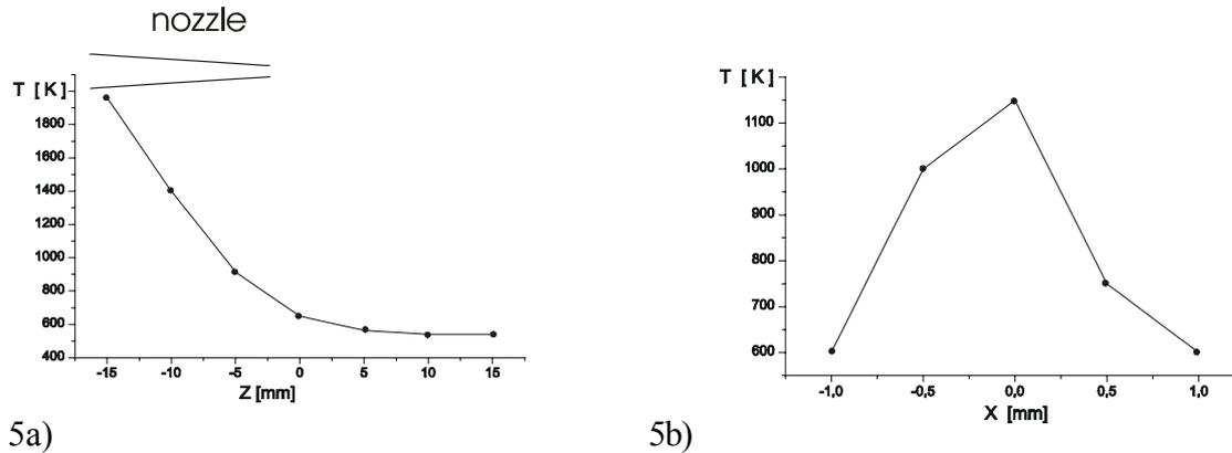
Figure 5: Axial temperature profile (fig. 5a) and radial temperature profile (fig. 5b) near nozzle orifice at 800 W microwave power.
