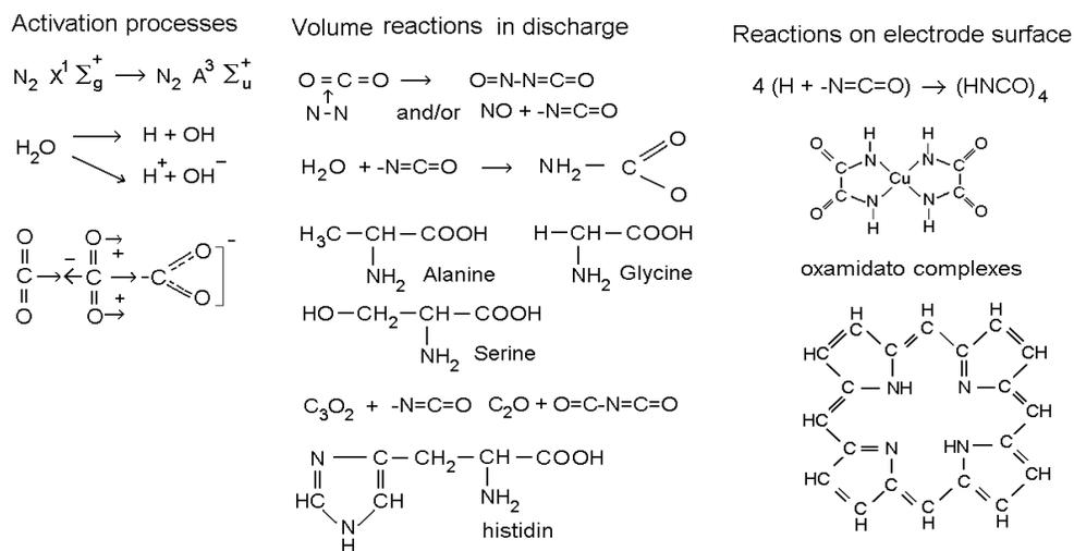
Fig.4 The overview of processes representing conversion of combustion exhaust in electric discharge and formation of amino acid condensation product and catalytic active spots on the electrode surface.
