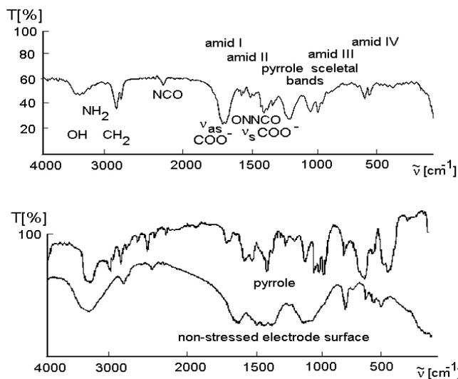
Fig.1 IR absorption spectra of solid condensation product, electrode surface and liquid pyrrole
