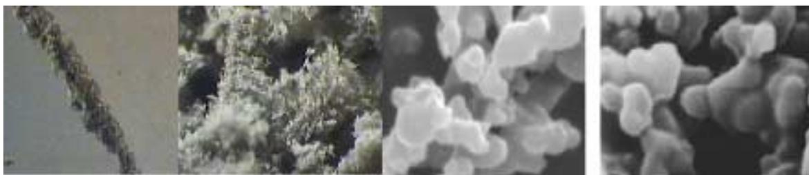
Fig.3 Left part of figure is microscopic photograph of solid product; magnification on left side 150 in middle 500 and on right side SEM photograph with magnification 8000; Right part of figure is SEM photograph of proteinoid protocells published by A.Pappelis & S.Fox [3]
