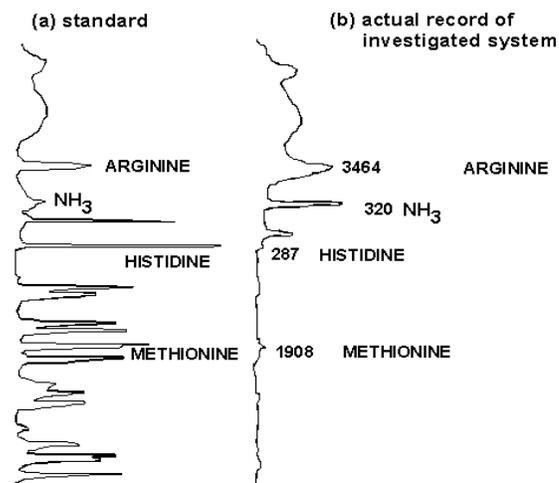
Fig.2 HPLC spectrum of product after conditioning in 6 molar HCl for 24 hours
