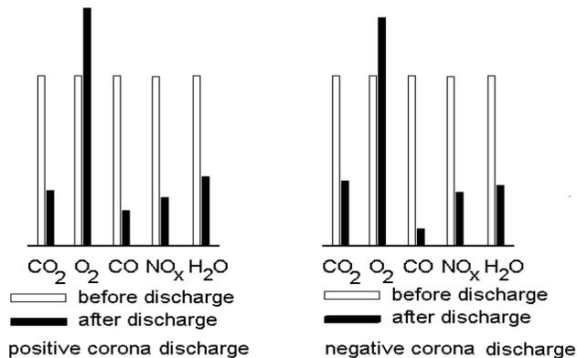
We have evidence for oxygen formation. In our experimental flowing system we have generated in this way from oxygen free combustion exhaust 5 and more % of oxygen after discharge system as we see from Fig. 6. Detail are in [2].
