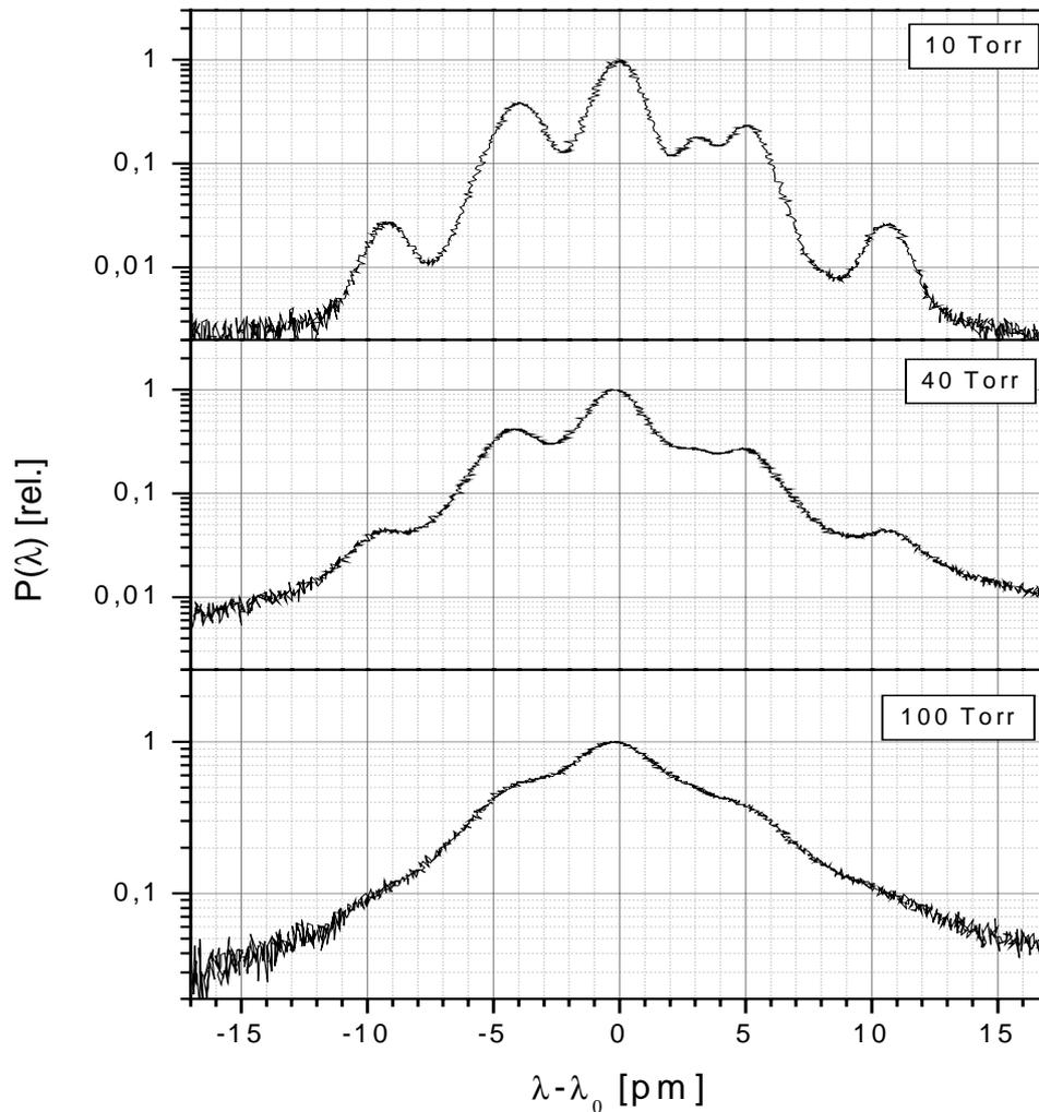
Figure 3: Normalized line profile of the  $6s[3/2]_2 - 6p[3/2]_2$  transition at 823 nm in xenon for 3 gas pressures.
