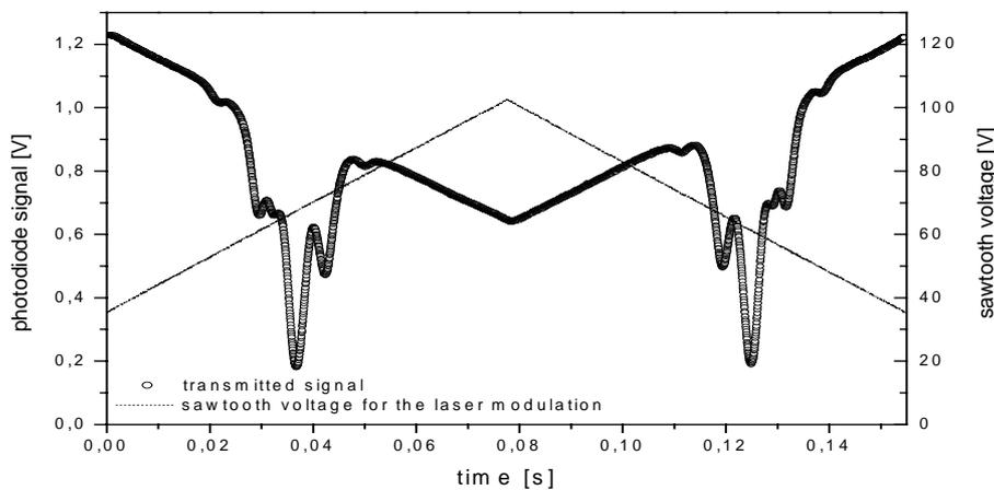
Figure 2: Absorption spectra of the  $6s[3/2]_2 - 6p[3/2]_2$  Xe transition at 30 Torr xenon and 1 mA and the temporal behavior of the sawtooth voltage controlling the laser modulation.
