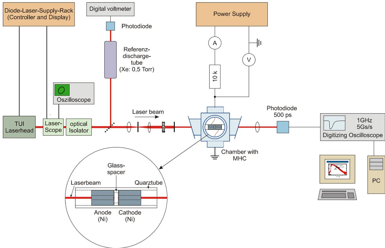
Figure 1: Experimental setup used to measure the absorption in a miniaturized hollow cathode discharge.
