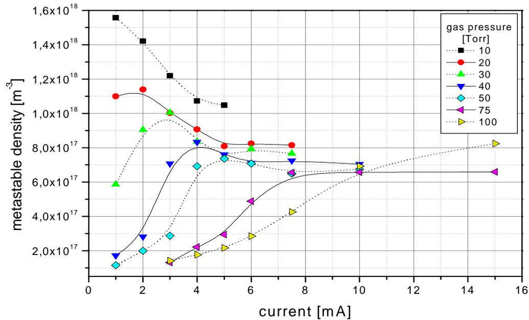
Figure 4: Development of population densities of the  $6s[3/2]_2$ -state of xenon, depending on discharge current and gas pressure.
