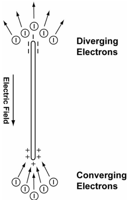
Figure 6: Illustration of polarity asymmetry for a long thin conductor in an electric field. Mobile electrons are convergent on one end and divergent at the other.
