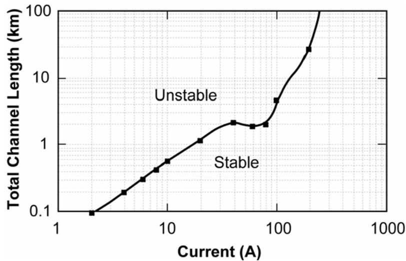
Figure 14: Stability diagram for a lightning channel represented by the equivalent circuit in Fig. 12. Unstable behavior with current cutoff to upper left of stability line; stable behavior with continuing current to lower right of stability line.
