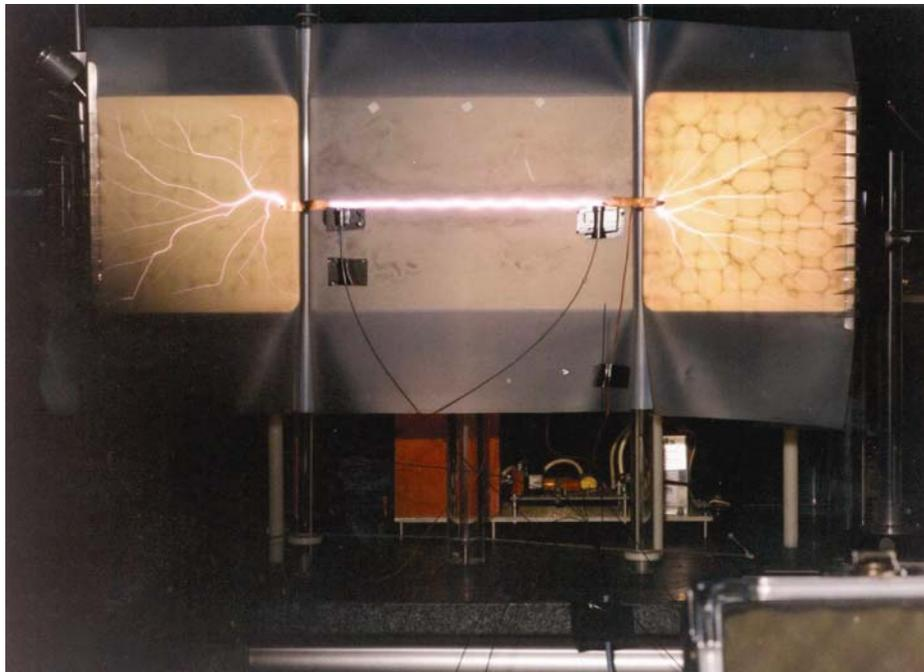
Figure 4: A double-ended tree linking positively and negatively charged surfaces in the laboratory.
