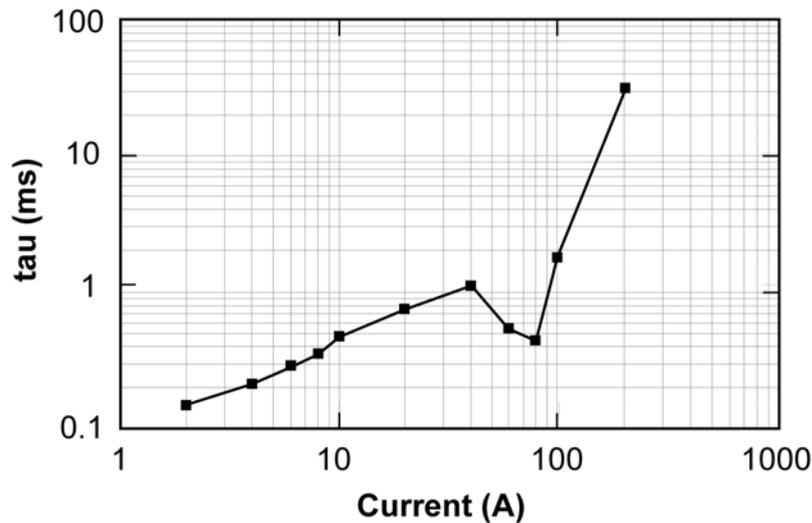
Figure 13: The time constant  $\tau$  representing the e-folding time of an electric arc in series with a voltage source. Adapted from Frind (1960).
