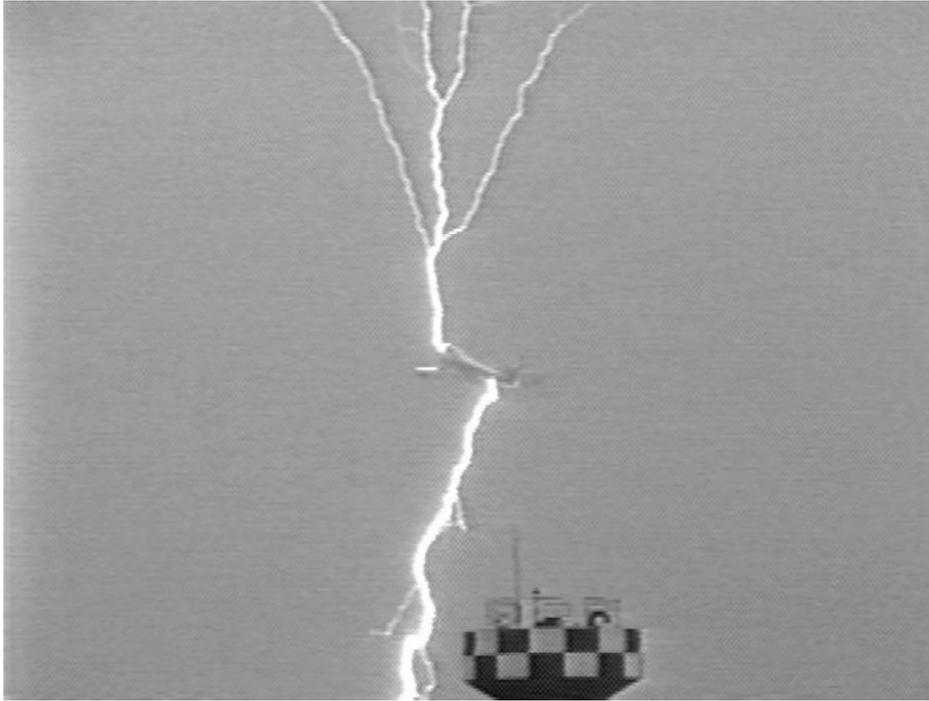
Figure 5: A double-ended lightning tree initiated on an airplane beneath a thundercloud. (Courtesy of Z. Kawasaki)
