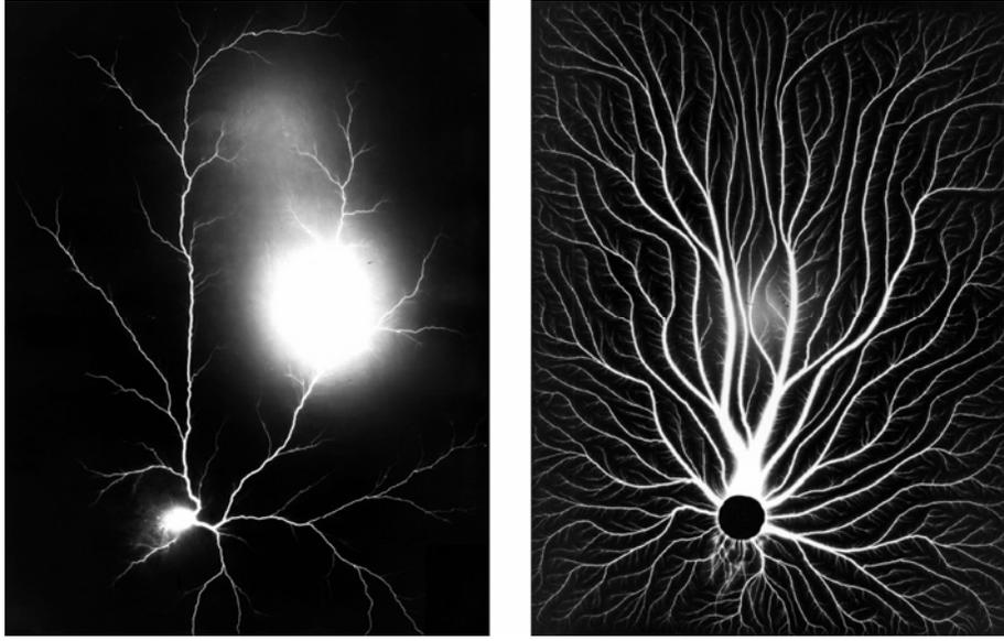
Figure 3: Surface discharges with a) positively, and b) negatively charged surfaces, showing marked contrast in structure.
