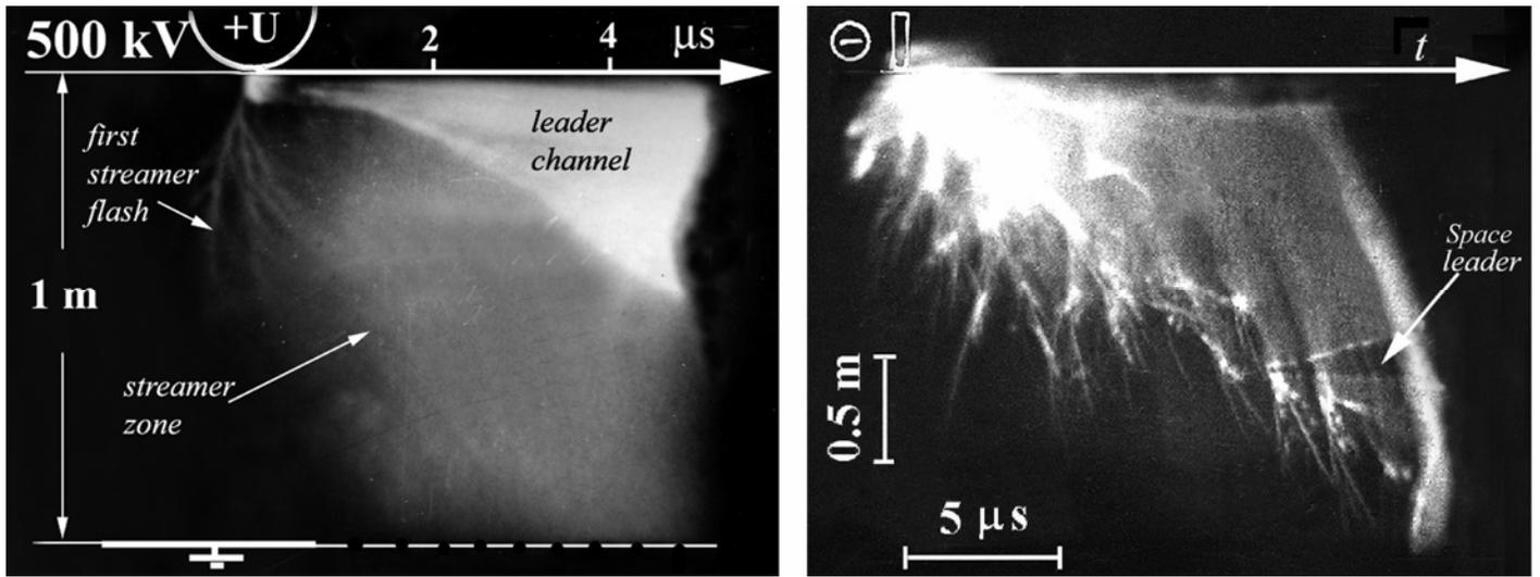
Figure 8: Streak camera imagery contrasting the extension of leaders with positive and negative polarity downward toward a ground plane. The positive leader progresses smoothly, whereas the negative leader is fitful and erratic.
