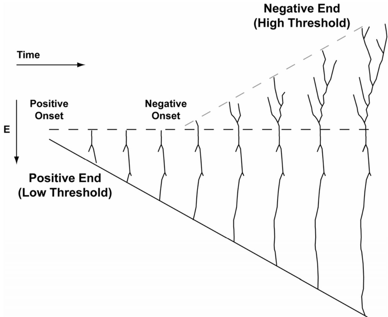
Figure 7: Schematic elongation of a bi-directional streamer/leader system, with positive polarity initiation, followed by extension of the negative end of the double-ended 'tree'.
