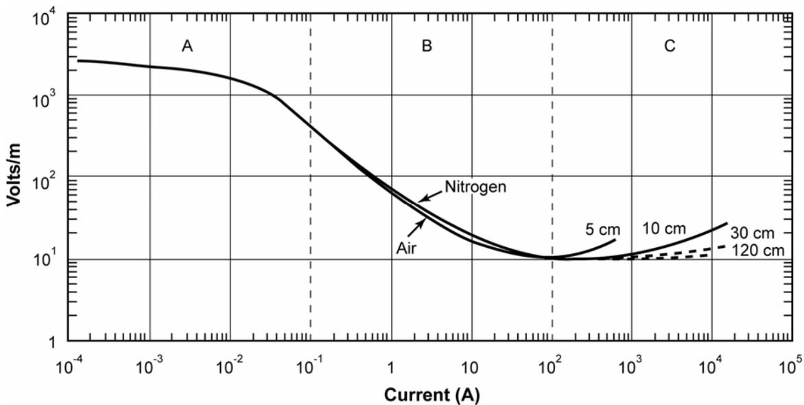
Figure 11: Current and voltage relationship for an electrical arc in air, showing negative differential resistance: the larger the current the smaller the resistance. From King (1961).
