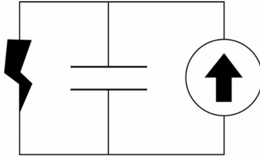
Figure 12: Equivalent circuit for a lightning channel to ground, analyzed by Heckman (1992). The continued extension of lightning into the charged cloud constitutes the current source  $I$ , the channel capacitance per unit length times the total channel length is the capacitor  $C$ , and the (non-linear) arc resistance per unit length times the total channel length is the total arc resistance  $R$ .
