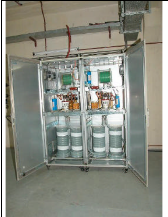
Fig.2 Assembly view of 50kW/120kHz push-pull oscillator
