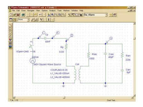
The model shows that the secondary resonates at 37.562kHz so I needed at adjust the primary inductor to 268.34uH to tune it. So I adjusted that and let it run.
