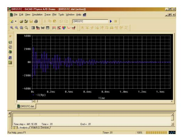
So not too bad!! The large inductor knocked the primary current down well. Thee primary voltage peaks at 14.77kV and the primary current at 240amps. If we set the quench time to 68uS we get a realistic situation.
