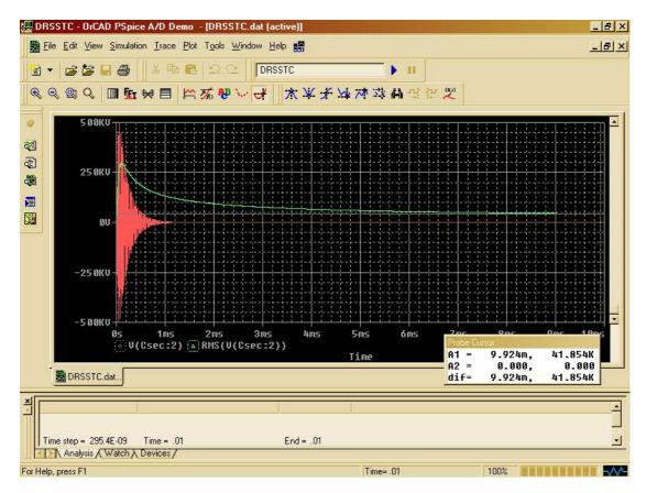
The real "key" to all this is to take into account the primary voltage, current, and frequency. If we have a primary frequency of 40kHz and want a peak current of 280 amps at 20kV. We really know the primary design.
