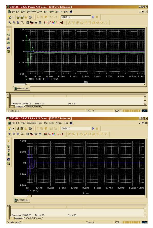
The primary RMS current for PRF of 100Hz is 31.57 amps:
