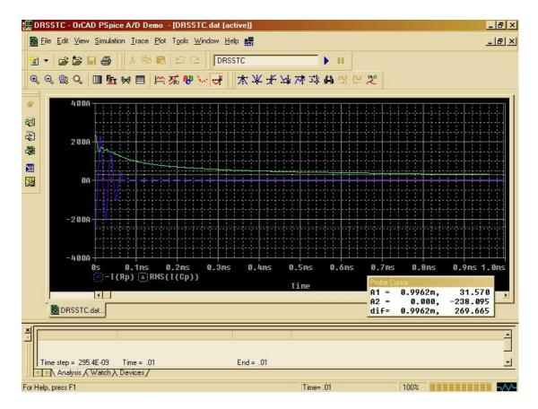
The RMS voltage to the load is 41.8kV. In a 220k ohm streamer, the power to the streamer is 7.942kW!! That suggests a streamer length of 160 inches!!
