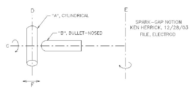
ELECTRODE B ROTATES AROUND AXIS E, SWEEPING PAST ELECTRODE A.
