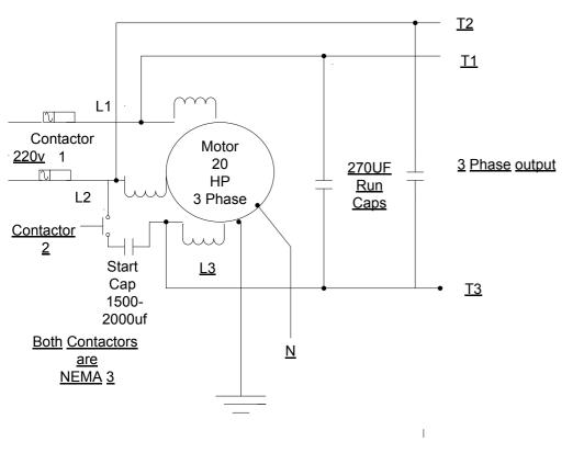
Both Contactors have 120 volt coils which will be transformer 220-120volt isolated. The Start Stop has DPDT with the Start switch held for motor startup then latched Stop open the latch releasing Contactor 1. Since the transformer is on both legs of 220v either open stops.
