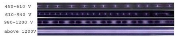
Fig. 4: Array of microdischarges in a 1D barrier discharge configuration in Ar/He [73]
