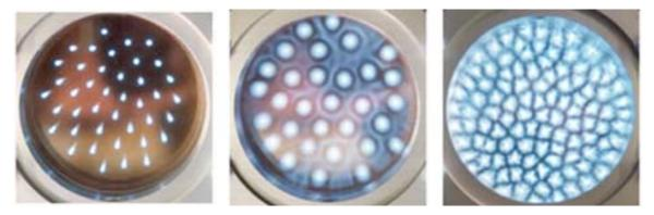
Fig. 5: Two-dimensional discharge patterns obtained in 5-mm quartz cell with planar walls filled with xenon/chlorine mixtures at different pressures (visible diameter: 8 cm)
