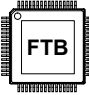
52-Pin LQFP-EP 0.65 mm Pitch 10.0 mm x 10.0 mm Body 7.0 mm x 7.0 mm Exposed Pad
