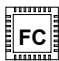
32-Pin QFN 0.65 mm Pitch 7.0 mm x 7.0 mm Body 4.7 mm x 4.7 mm Exposed Pad
