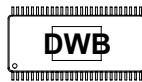
54-Pin SOICW-EP 0.65 mm Pitch 17.9 mm x 7.5 mm Body 6.3 mm x 4.6 mm Exposed Pad
