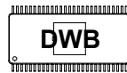
54-Pin SOICW-EP 0.65 mm Pitch 17.9 mm x 7.5 mm Body 4.6 mm x 4.6 mm Exposed Pad
