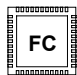
44-Pin QFN 0.65 mm Pitch 9.0 mm x 9.0 mm Body 6.7 mm x 6.7 mm Exposed Pad
