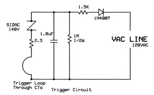
The AC line is simply rectified and charges a 1uF cap. At about 140 volts DC, the SIDAC fires and creates a powerful tight current pulse. This circuit is designed to fire at 60 Hz, but simply removing the 1N4007 will make it fire at 120 Hz.
