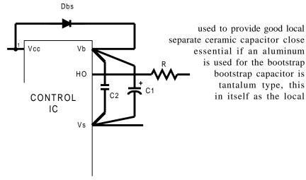
Fig 2) Recommended layout of the Bootstrap Components
