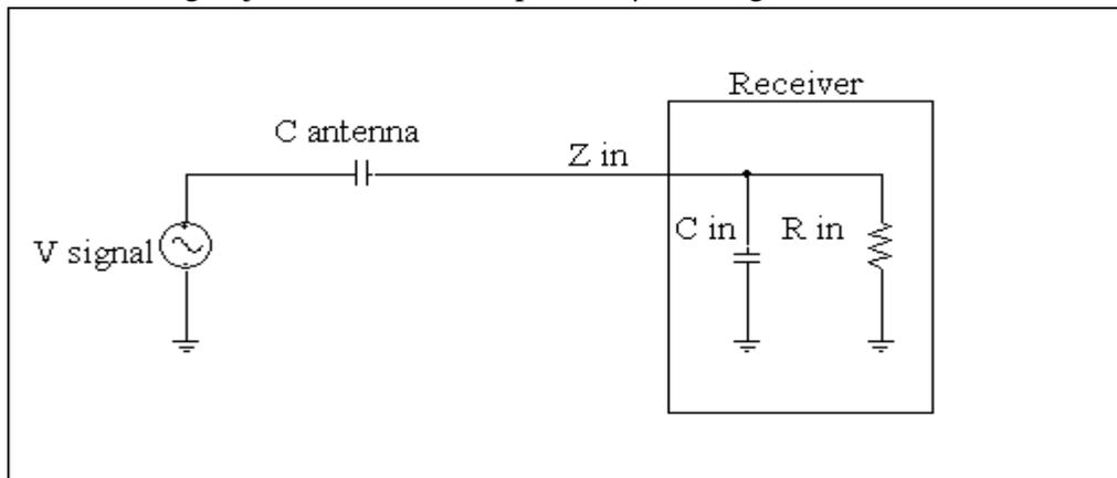
Whip antennas possess a theoretical isotropic capacitance of  $\sim 11$  pF/m. If the signal of interest is at 8 Hz, the source impedance becomes 900 megohms! To avoid loading the signal down, the receiver must present an input impedance that is an order of magnitude larger.
