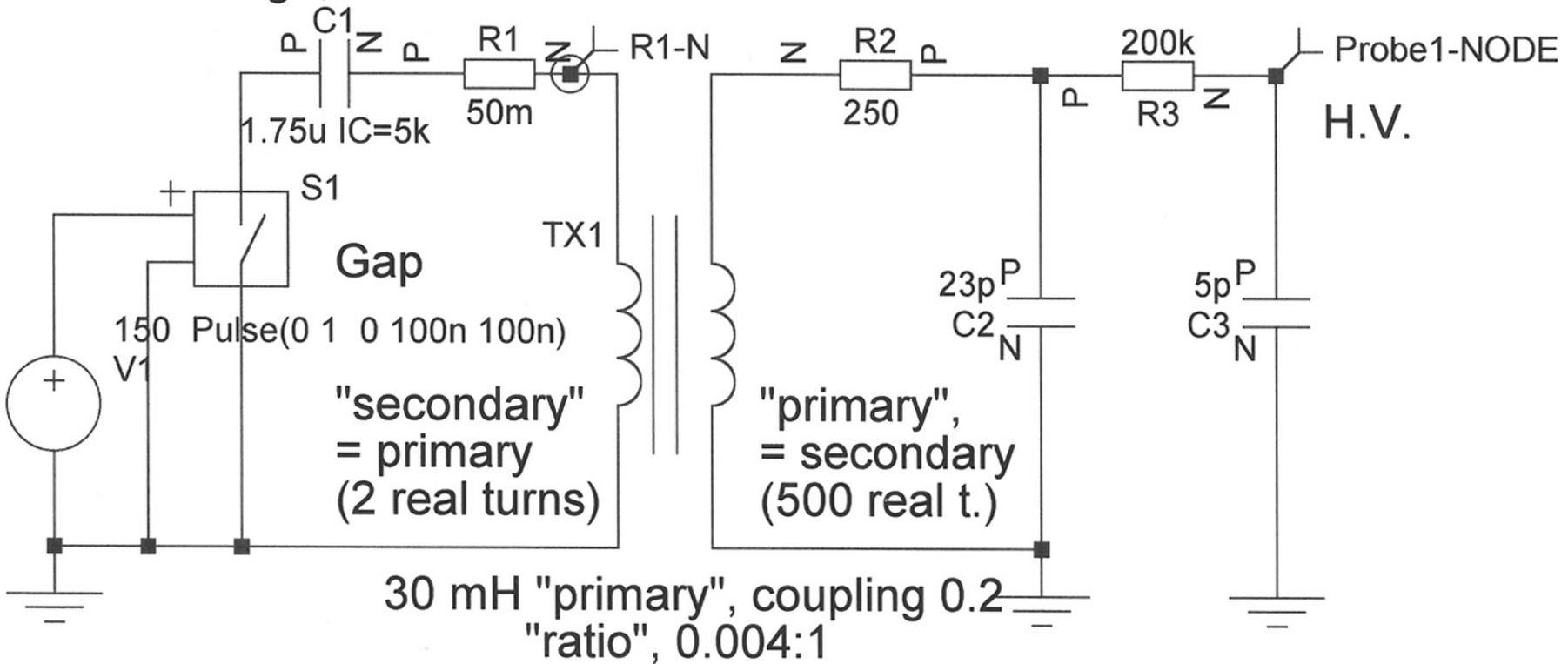
Simulation of a conventional Tesla coil utilizing a reversed-transformer component. Ken Herrick 5/17/03.
