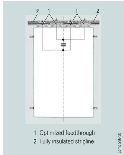
**Fig. 7 Optimum connection of a low-inductance MKK capacitor by a fully insulated stripline**
