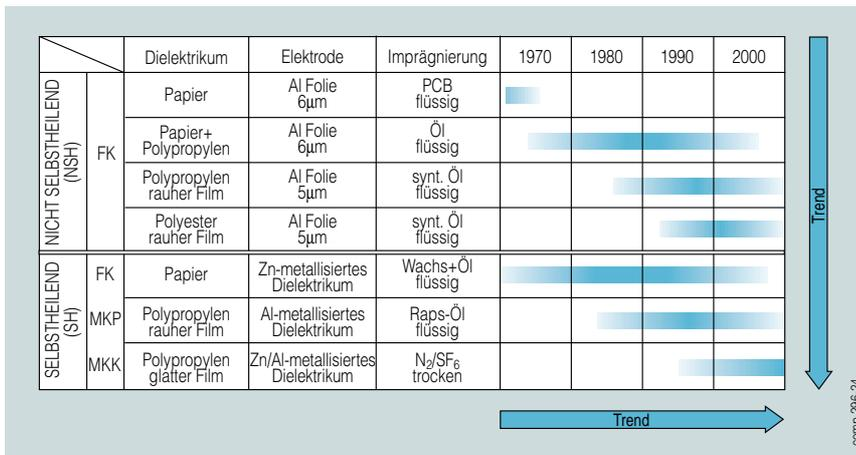
**Fig. 1** In capacitors for rail traction, the trend is moving away from non-self-healing to self-healing designs and from liquid to gas impregnation
