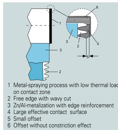
**Fig. 4 Combined wavy and smooth cuts increase the contact surface of MKK capacitors**
