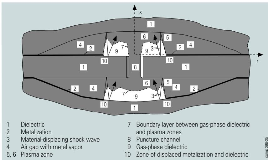
**Fig. 2** Self-healing puncture in a dielectric of organic material
