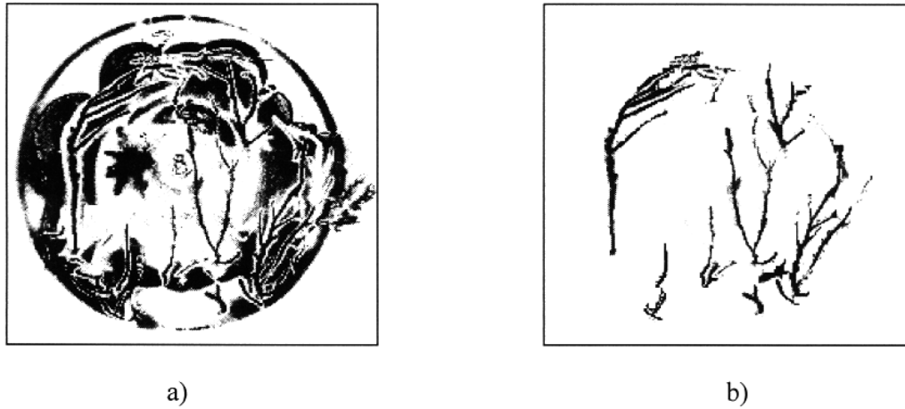
Figure 3. The electrostatic discharge structure for a poling time of 2.2 h. (a) the original structure and (b) the extracted channel structure ( D = 1.36 \pm 0.02 ).
