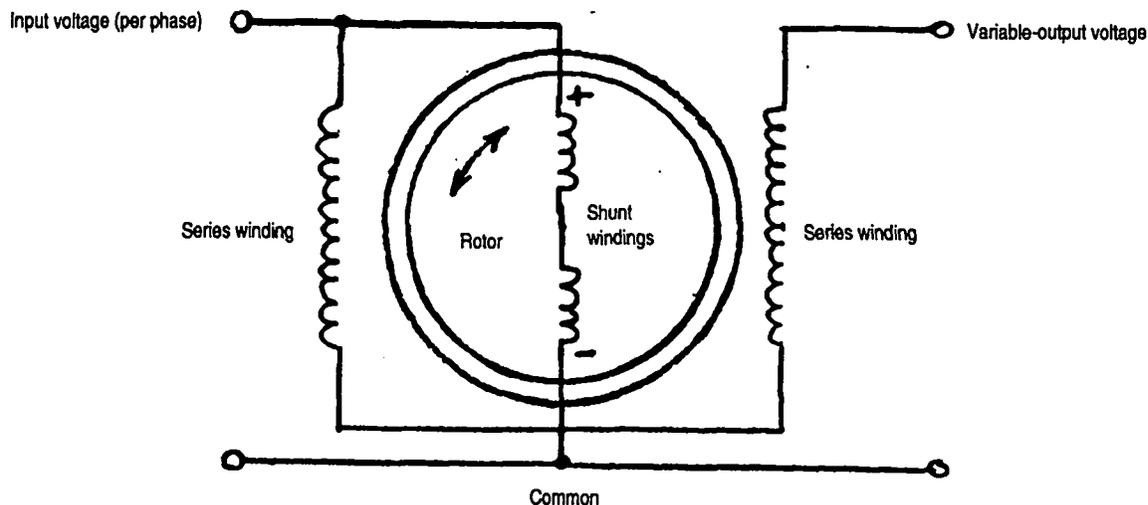
Figure 15-11. The induction voltage regulator (IVR).
