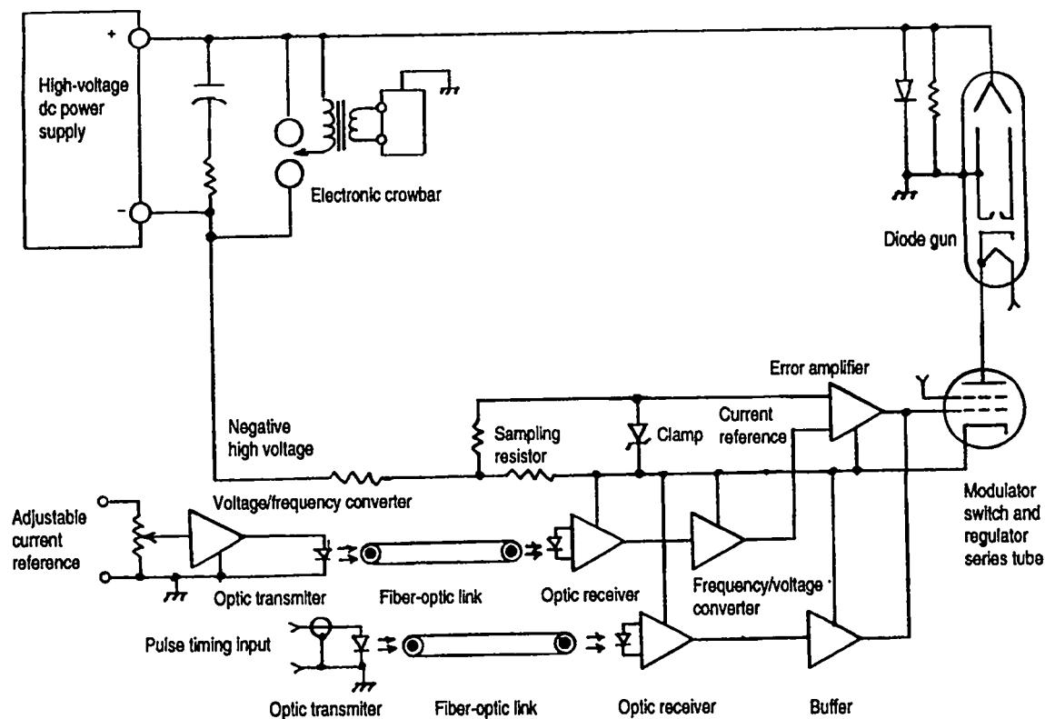
Figure 16-6. Modulator switch and pulse-current-regulator tube in series with high-voltage bus.
