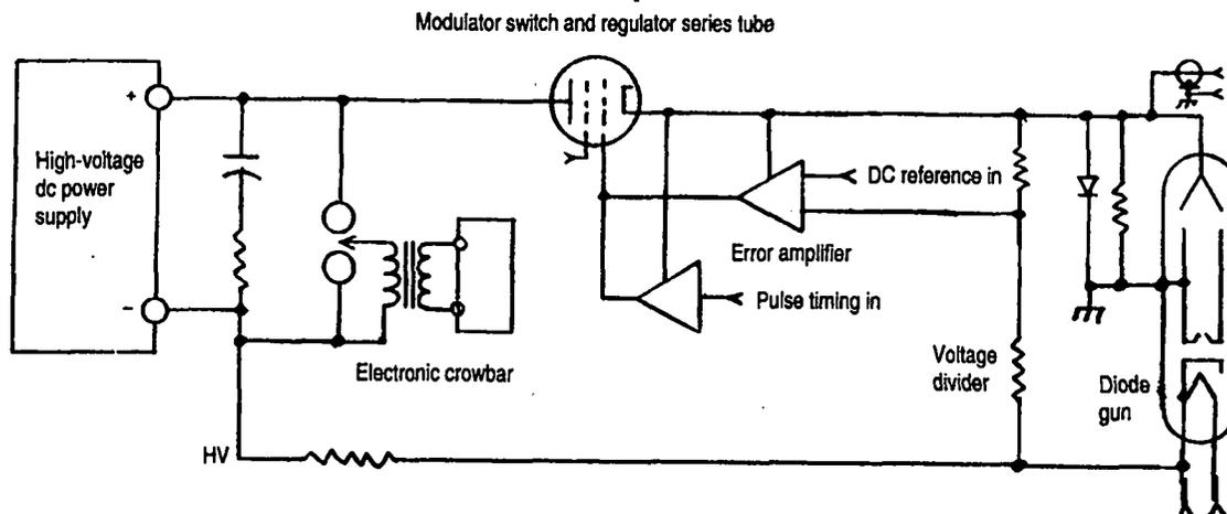
Figure 16-4. Modulator switch and regulator series tube in positive return of high-voltage power supply.
