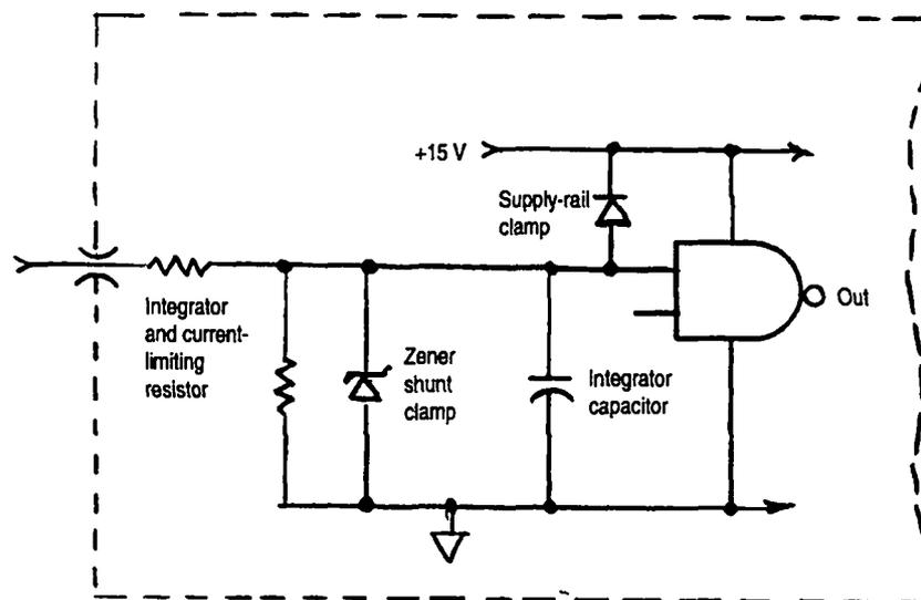
Figure 20-6. Methods of protecting integrated-circuit inputs.
