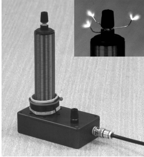
**Figure 3.** A small continuously driven Tesla coil system operating at a frequency of approximately 4 MHz. The inset photograph shows the corona produced when the coil draws approximately 36 W of power.
