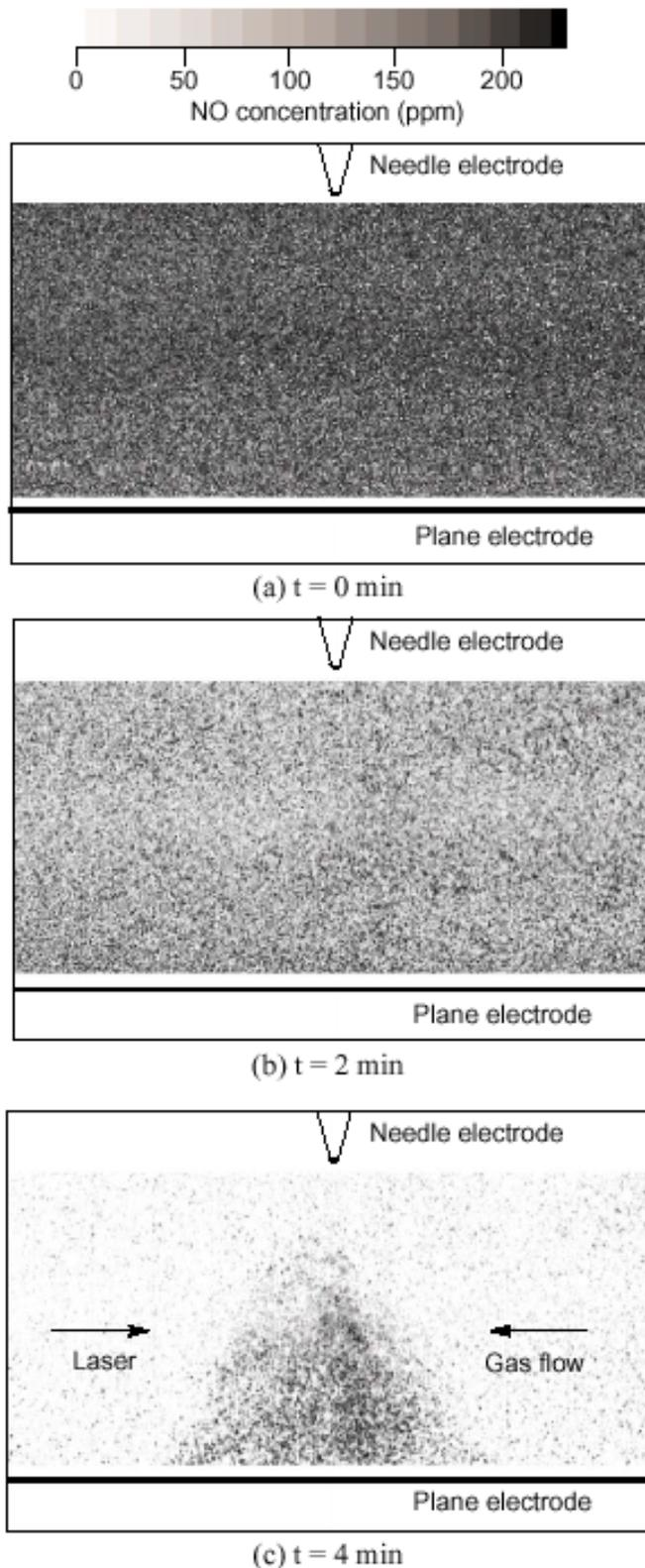
Fig. 3. Time evolution of the NO LIF image during the streamer corona discharge in the closed system. Time  $t=0$  min and  $t=4$  min indicate the start of the discharge and the steady-state, respectively. Operating gas: NO (200ppm)/air, flow rate 1L/min, applied voltage: 21kV.
