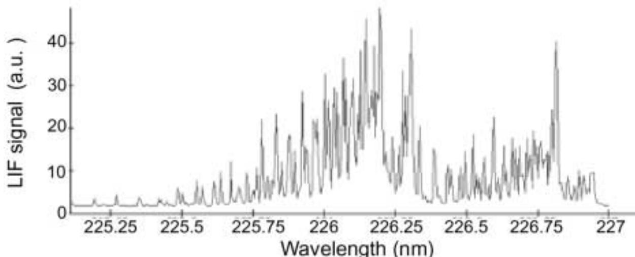
Fig. 2. LIF spectrum of NO molecule. Operating gas: NO (300ppm)/air.
