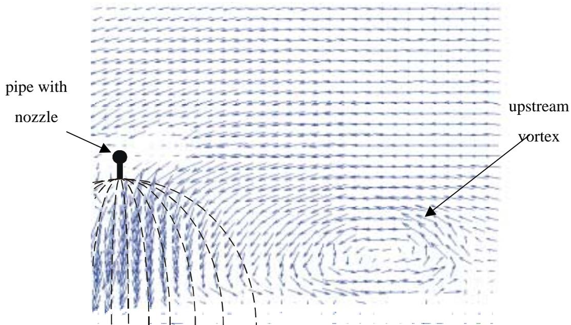
Fig.4. Velocity field of the gas flow at the upstream side of pipe with nozzle electrode during corona discharge. Operating voltage +35 kV, current 120 mA, gas mean velocity 0.56 m/s, lower plate electrode grounded.
