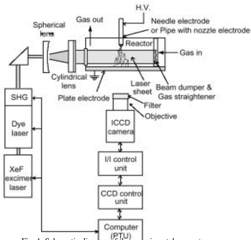
Fig. 1. Schematic diagram of the experimental apparatus.
