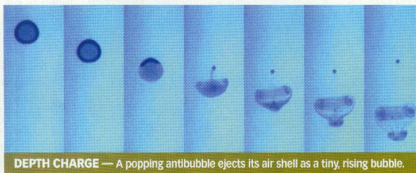
DEPTH CHARGE — A popping antibubble ejects its air shell as a tiny, rising bubble.
