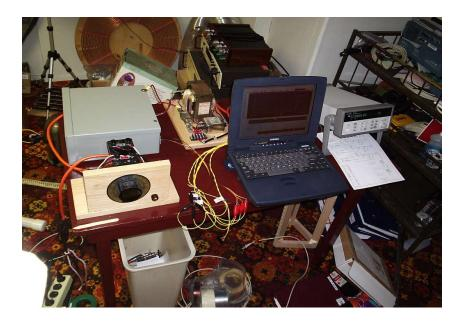
The goal was to see how long the dielectric would hold up to ionization at the edges of the plates which is the limiter.
