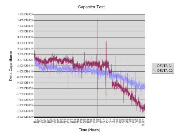
At about the 75 hour mark, the capacitance started to drop at an obvious faster pace and ended up at about 1% lower than the 20 hour mark. This is very likely due to internal arcing. Both capacitors seem to degrade at about the same time and pace. Capacitor #2 also had "something" happen at 45 hours but it did not seem to really hurt anything.
