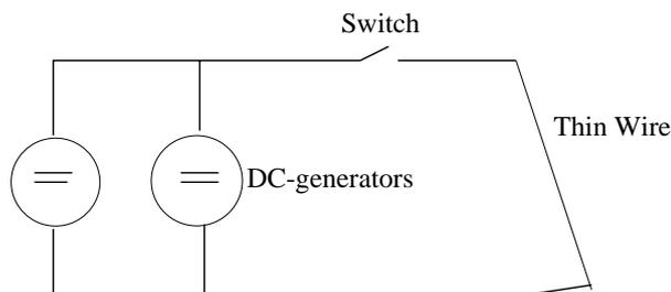
Figure 2.1: Nasiłowski's circuit for the creation of wire fragments.
