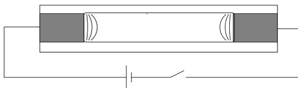
Figure 2.10: Agitation at the interface between solid and liquid metal.
