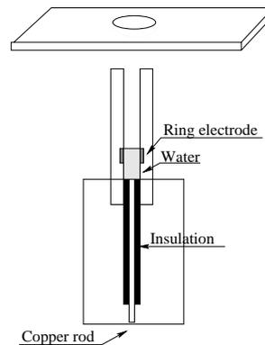
Figure 5.2: Punching of metal with water-arc explosions.
