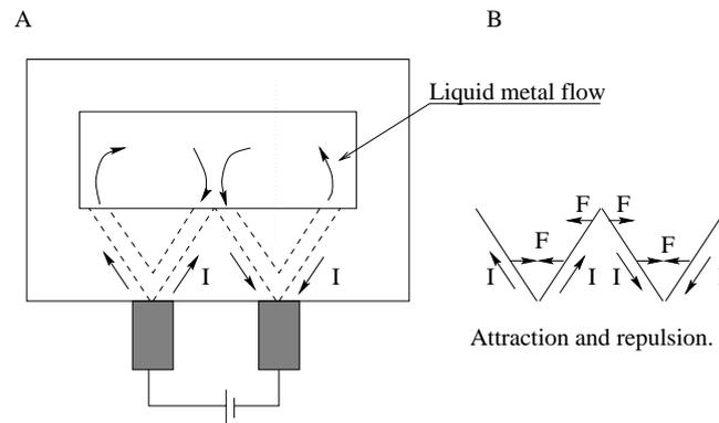
Figure 5.1: (A) Hering's liquid metal pump. (B) Seat of forces.
