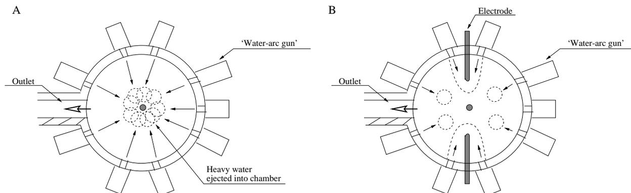
Figure 5.5: Plasma fusion chambers. (A) Impact fusion, (B) Impact fusion and arc-discharge fusion.
