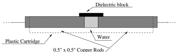
Figure 2.17: Experiment to create powerful water-plasma explosions.
