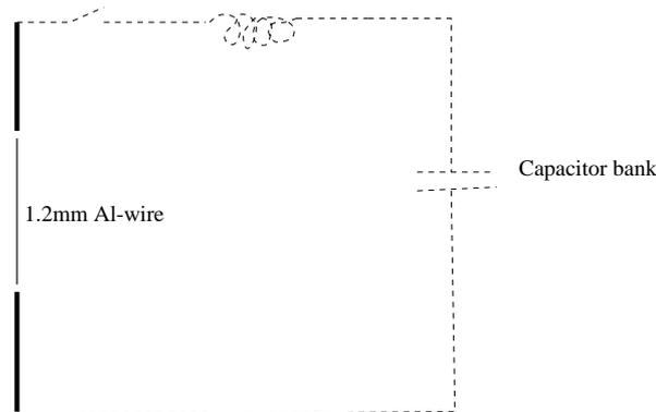
Figure 2.5: Graneau's experimental setup for wire fragmentation.
