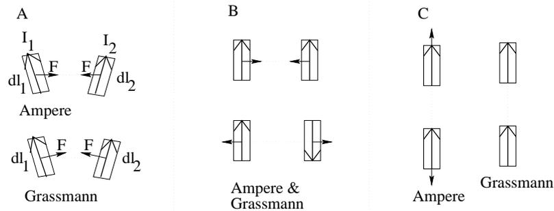
Figure 3.1: The forces between two current elements according to Ampère's and Grassmann's equations. (A) Forces between current elements. (B) Transverse forces between parallel elements. (C) Longitudinal forces between co-linear elements
