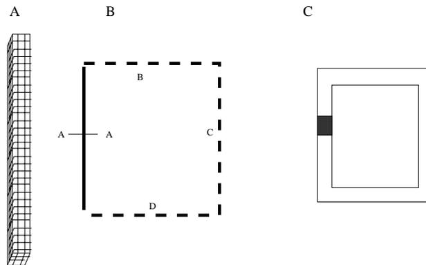
Figure 3.3: (A) Subdivision of a straight conductor. (B) Omitted parts. (C) Small segment of a circuit.
