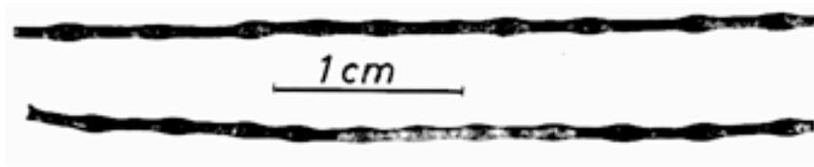
Figure 2.4: Unduloids formed by surface melting and pinch pressure. From Jan Nasilowski, Instytut Elektrotechniki, Warsaw, Poland.
