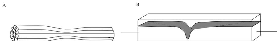
Figure 1.3: The pinch effect. (A) As ‘like currents attract’, the conductor squeezes itself radially inward. If the material is too weak to sustain the pressure it is pinched off at some point. (B) Pinch depression in a liquid conductor, caused by a current of some hundred Amperes.
