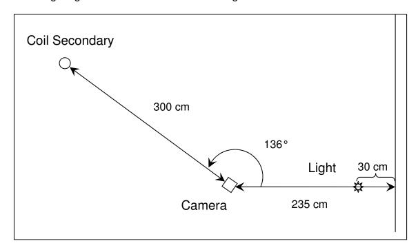
In the low light setting, the illuminance measured at the secondary (at camera height of 150 cm) was 9 lux.
