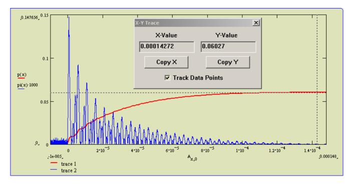
The power and energy graph shows that the total energy expended is 60.3mJ. The original capacitor energy was 63.3mJ. The primary capacitor's ESR is rated at 0.005 ohms and the coil's ESR is measured at 0.0217 ohms with a less than trusted meter. If we calculate the equivalent resistance of the gap, it is 0.54 ohms. Typical spark gaps are usually in the 3 ohm range so the gap seem to be very efficient.
