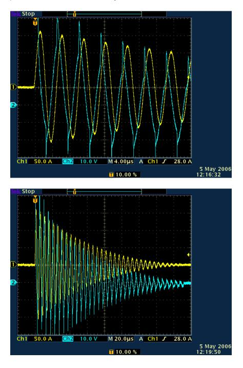
If we divide the voltage waveform but the current waveform, we can see the instantaneous resistance across the gap.
