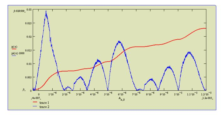
The instant power (blue) is the power expended every 4nS in milliwatts. The red line is the energy lost in Joules. The time scale is identical tot he first graph. In this case, one may simply note that the energy loss during the gap's initial turn on is reasonably close to the normal full on operation of the gap.
