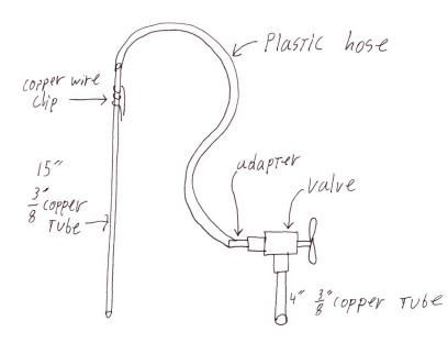
The siphon consists of a 15" copper dip tube with a mine dip to hold it to the side of a bucket in the proper popition. A 5 foot plastic hope goes to a brass adapter to a brass value with a short copper tube. The siphon is used in spanging, cooling, raching and bottling. The parts can be purchased at a good hardware store (7\$10).
