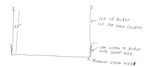
The bottom is cut off of a plastic bucket and screen wire is sewn to the bottom to make a seive. The screen to must be sewn well to hold the weight of the wet grain
